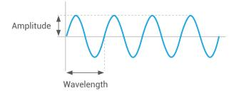
Wavelength and frequency are inversely related. Increasing the frequency will decrease the wavelength, which is good for resolution. But there is a trade off: with increased frequency, penetration will also decrease.
